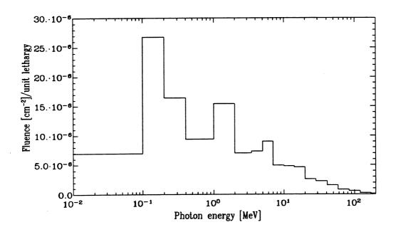
Figure 6: Top: Spectrum of photons produced in the whole system and initiating electromagnetic cascades, normalized per one 100-GeV proton. Bottom: Fluence of cascade photons emerging from 1 m concrete shield, per cm² and per one 100-GeV proton, averaged over regions 12, 18, and 24. Target diameter 2 cm.
