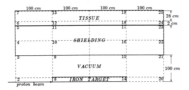
Figure 2: Cylindrical geometry model of the shielding arrangement assumed for calculations. Solid lines are material boundaries, dashed lines are region boundaries; region numbers are indicated in top right or left corners.
