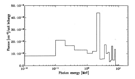
Figure 5: Fluence of photons from capture of thermal neutrons and inelastic interactions below 20 MeV emerging from 1 m concrete shield, per cm<sup>2</sup> and per one 100-GeV proton, averaged over regions 12, 18, and 24. Target diameter 2 cm.
