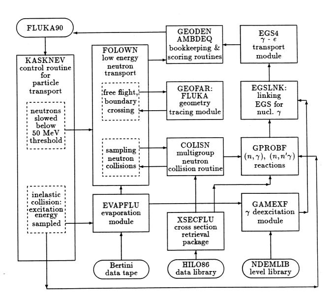
Figure 1: Simplified flow diagram for sampling of low energy neutrons and photons of nuclear origin in the FLUNEV code.
