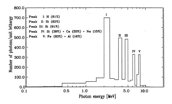
Figure 4: Spectrum of photons produced by thermal neutron capture in concrete, normalized per one 100-GeV proton. Target diameter 2 cm.
