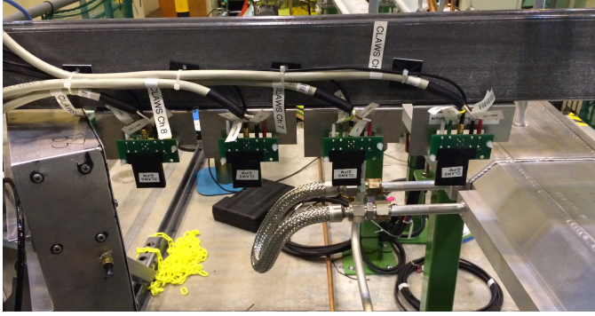
Figure 21: Photograph of the backward CLAWS station installed in the BEAST II system taken from the position of the IP. Four CLAWS detectors are mounted on the BEAST frame in the plane of the accelerator with increasing radial distance from the beam pipe, which is shown on the right. On the left, one of the Crystals boxes as discussed in Section 3.4 can be seen.
