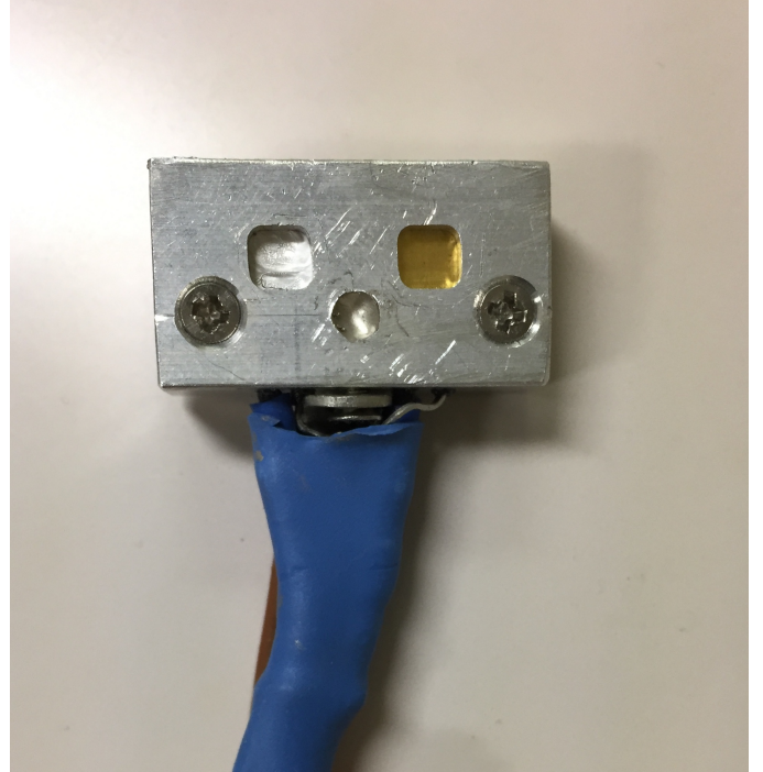
Figure 2: A PIN diode module containing two diodes and a thermocouple. The active area of the diodes is exposed, showing the aluminum foil covering one and the gold foil covering the other to reduce the X-rays from synchrotron radiation.
