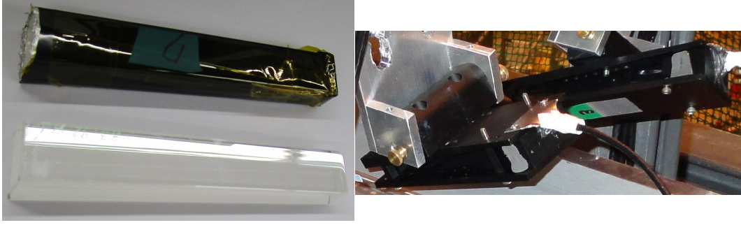
Figure 17: Left: a BGO crystal with (top) and without (bottom) the wrapping material. Right: the BGO crystals with the supporting structures.
