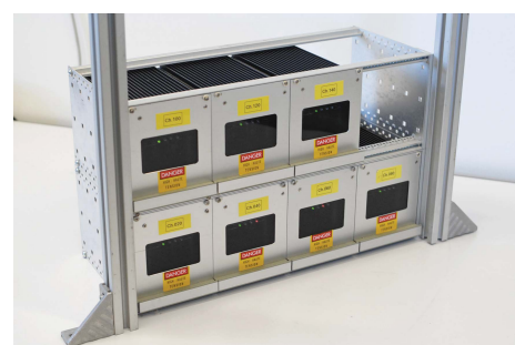
Figure 4: Seven picoammeters assembled in a mini crate.
