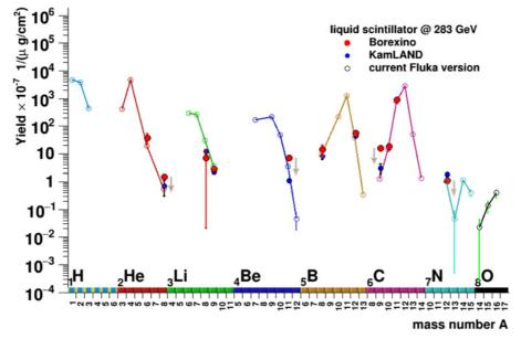
**Figure 5.** Muon-induced cosmogenic isotope production yields in liquid scintillator underground detectors, assuming realistic muon spectra with 283 GeV average energy. Experimental results from Borexino [22] and KamLAND [23] are shown by the red and blue symbols respectively: when present, arrows indicate an upper limit. Preliminary predictions obtained with the current version of FLUKA for the measured isotope production rates are shown by the open symbols.
