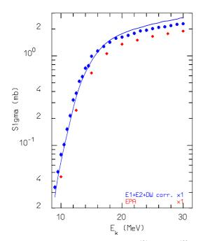
**Figure 3.** Electronuclear cross section for  ${}^{181}\text{Ta}(e^-, n){}^{180}\text{Ta}$  as a function of  $e^-$  energy in the few-tens of MeV range. Blue dots are experimental data from [16], red dots are FLUKA simulations with EPA, the blue line are FLUKA results with the full approach described in the present paper.
