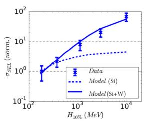
**Figure 11.** Single Event Effect cross section as measured at CHARM (symbols) and predicted by FLUKA without and with heavy materials, as a function of the spectral hardness.
