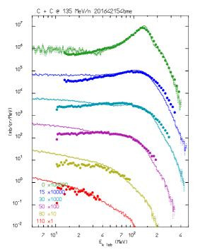
**Figure 8.** DDCX C(<sup>12</sup>C,xn) at 135 MeV/n as a function of energy for various angles (indicated in figure). Symbols: exp. data [29], histograms: FLUKA with the modified BME.
