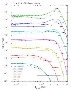
**Figure 6.** DDCX C(<sup>14</sup>N,xn) at 400 MeV/n as a function of energy for various angles (indicated in figure). Symbols: exp. data [30], histograms: FLUKA with the previous RQMD version.
