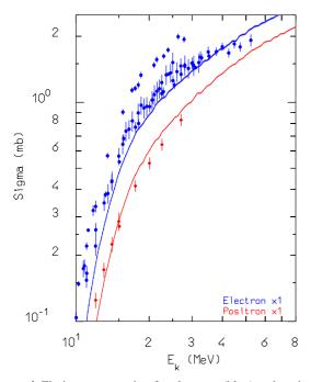
**Figure 4.** Fission cross section for electrons (blue) and positrons (red) on  $^{238}$ U as a function of electron energy. Symbols: experimental data from [18–20], lines: FLUKA EMD.
