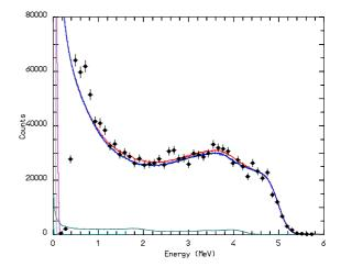
**Figure 10.** Pulse height spectra for a BC505 liquid scintillator cell with 8.9 MeV incident neutrons. Black symbols: exp. data [32], colored curves: simulated response accounting for quenching and energy resolution. Red curve: total response, blue: proton contribution, light blue: deuterons, purple: alphas, dark green: electrons, grey: heavy recoils.
