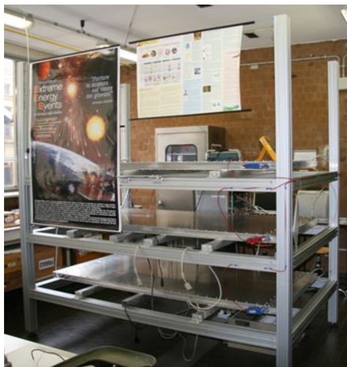
Figure 4. One EEE Project telescope located at Liceo Classico Massimo D'Azeglio in Turin, composed of three MRPC chambers.
