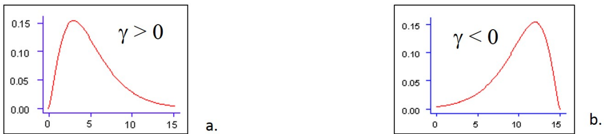
Fig. 23: Examples of asymmetric particle beam distributions with positive (a) and negative (b) skewness values
