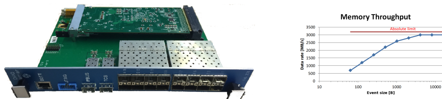
Figure 1: Data Handling Card (DHC) mounted on a VME carrier card (left) and data throughput as DHCsw as a function of event size (right)
