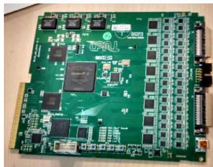
Fig. 3: Picture of a 64 channels uTCA digitization card for the ionization charge readout
