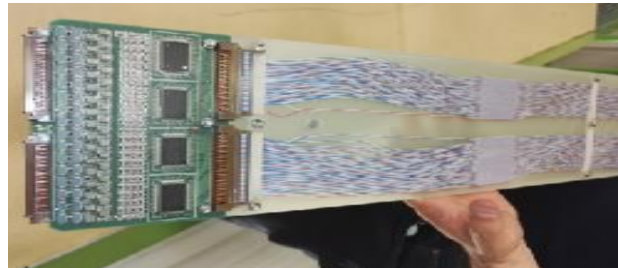
Fig. 2: A front-end card with 4 cryogenic ASIC amplifiers mounted on a supporting blade for insertion in a chimney
