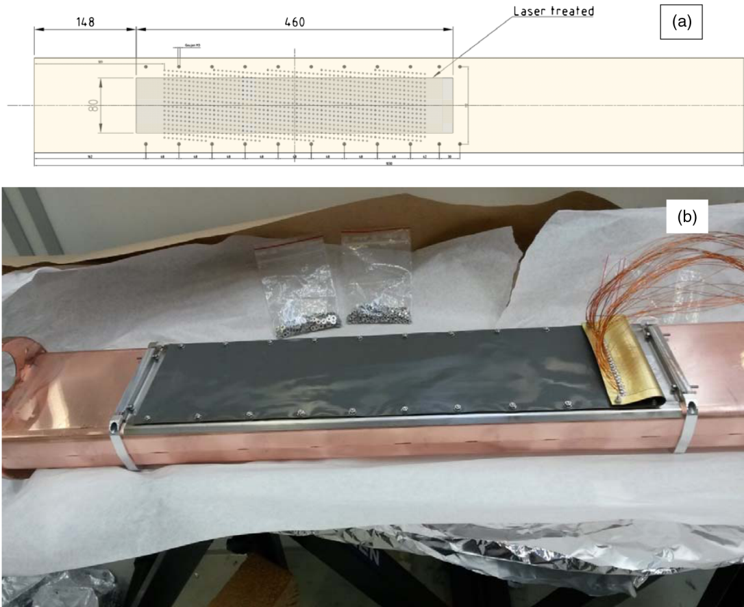
FIG. 2. (a) Schematics of the laser treated region on the top half of the liner; the bottom half is treated symmetrically. (b) One of the finished liners assembled with the stripline monitor before installation in the SPS magnet.
