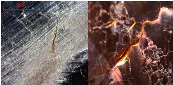
Figure 4: Microscopic pictures of the copper cavity substrate at the reception.
