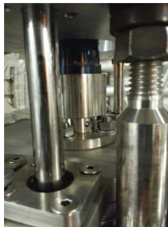
Figure 3: Picture of the unscrewed “goupille” which caused the fall of the TDI upper jaw in IR 2.
