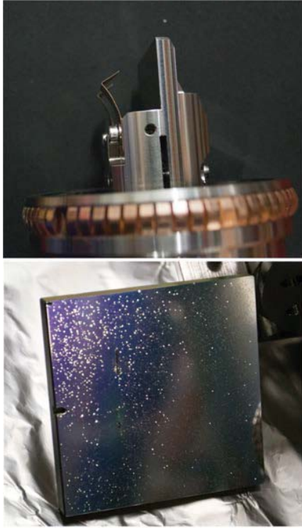
Figure 3: BSRT mirror holder clamps deformation and coating blistering, as evident after the B2 system removal in September 2012.
