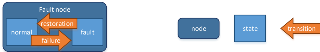
Fig. 9: A fault node with normal and fault states and failure and restoration transitions
