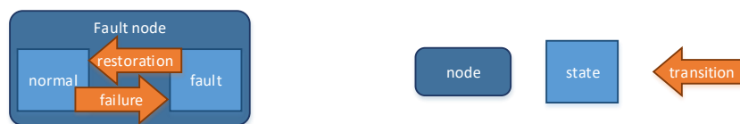
Fig. D.1: A fault node with normal and fault states and failure and restoration transitions
