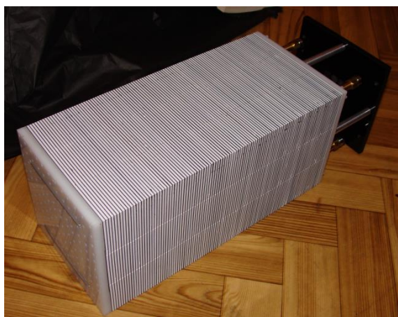
Figure 4. Calorimeter part of the module (unsealed).
