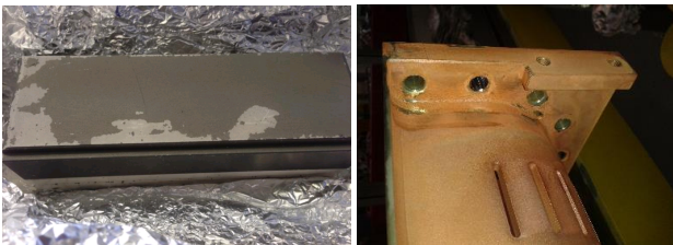
Figure 3: Issues with coatings in LS1: damaged Ti/NEG/Cu/NEG coating on hBN block due to hBN outgassing during bakeout (left) and discolored copper coating on beam screens due to Cl contamination (right). Photos courtesy of M. Taborelli and A. Perillo Marcone.
