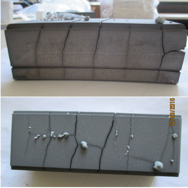
Figure 4: Cracked hBN blocks after thermal treatment in vacuum at 800°C. Material projections are visible on the block surface.
