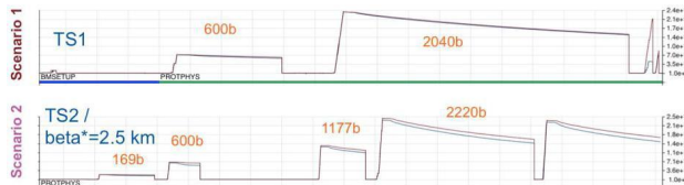
Figure 2: Ramp-up of the intensity after short stops from nominal operation without (scenario 1) and with (scenario 2) massive hardware interventions. The first was for example applied after technical stop one (TS1), the latter after technical stop two (TS2) followed by the \beta^* = 2.5 km run.
