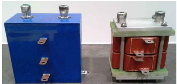
Figure 1: The currently used anode resistor (right) and the newly developed replacement resistor (left).
