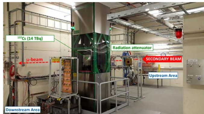
Fig. 2. GIF ++ facility irradiation area.
