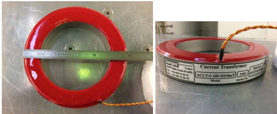
Figure 6.37: Picture of the MYRRHA LEBT AC Current Transformer procured by Bergoz Instrumentation, France.
