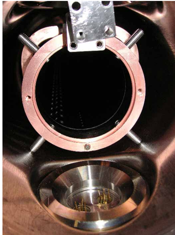
Figure 9.6: Picture of 2014 COLDEX a-C coated beam screen during re-installation. Courtesy of G. Bregliozzi.
