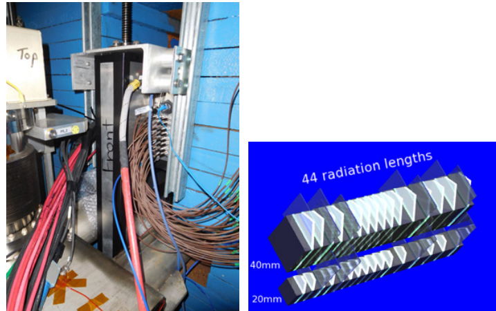
Figure 1. Left: a photo of the RHICf detector installed at 18 m from the STAR interaction point in the RHIC. Right: schematic view of the RHICf calorimeters.
