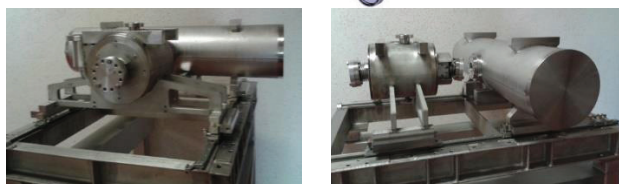
Figure 3: the test bench with a dummy cavity and solenoid.
