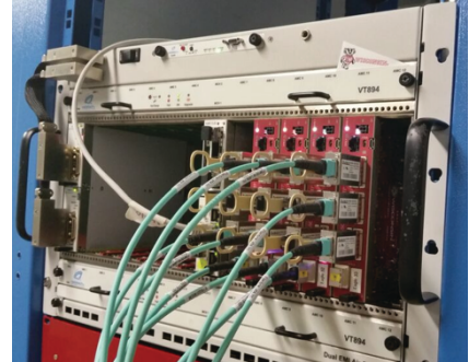
Figure 5. Schematic overview (left) and image (right) of the tracklet demonstrator system. The stub source and track sink are on the same processing board. Estimated data transfer rates between the boards are also shown.
