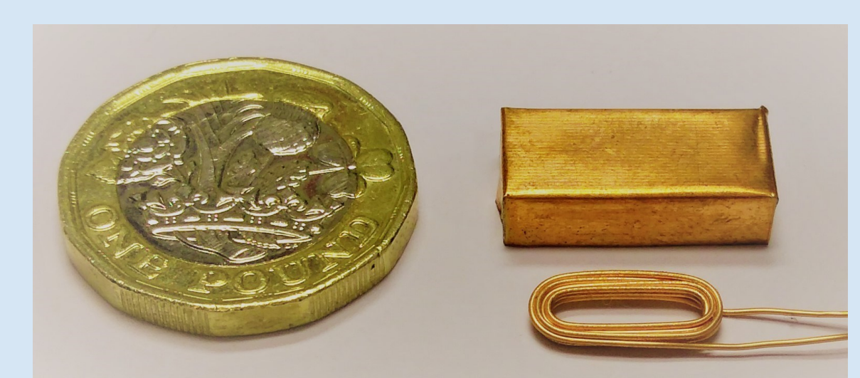
Prototype Shield Box with coil, box dimensions: 18 x 8 x 4.5mm
