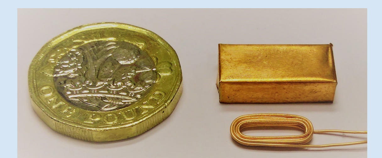
Prototype Shield Box with coil, box dimensions: 18 x 8 x 4.5mm
