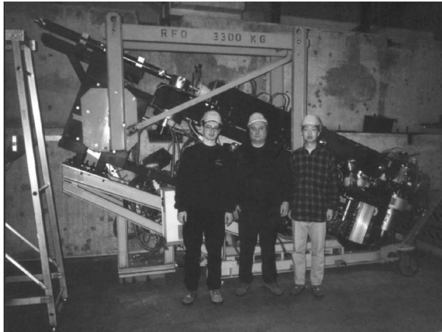
Figure B.1: Photograph of the RFQ system taken prior to its transfer to the storage area. The beam pipe and the most downstream cryopump have already been removed. Standing in front of the system are members of the Caltech group involved in the RFQ dismantling, from left: M. Gataullin, S. Shevchenko, and X. Lei.
