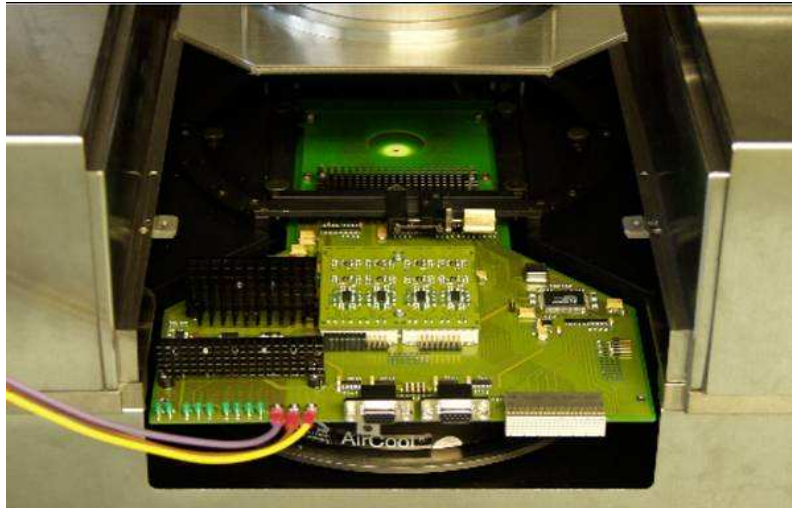
Figure 5.1: The PPrASIC test-hardware mounted in the wafer-probe station.
