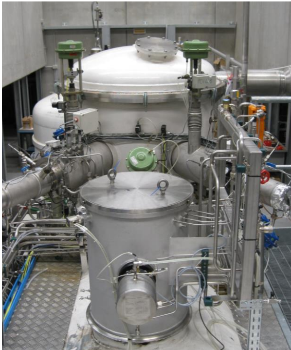
Figure 2. The top view of the ALPI refrigerator is shown, with its expansion turbines: the supercritical turbine is the one on the front.
