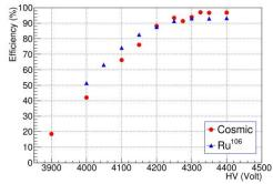
**Fig. 5** Efficiency variation as a function of HV for cosmic muons and <sup>106</sup>Ru-Rh source.
