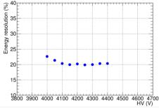
Fig. 4 Energy resolution as a function of HV.
