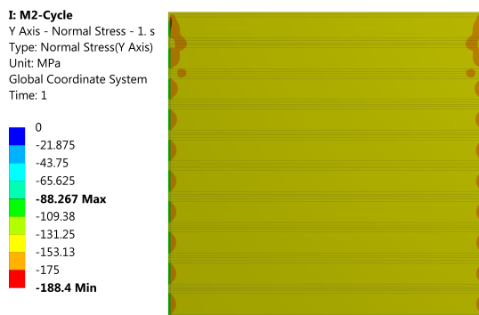
Figure C.1: Vertical loading of the M2 10-Stack model to 150MPa in compression
