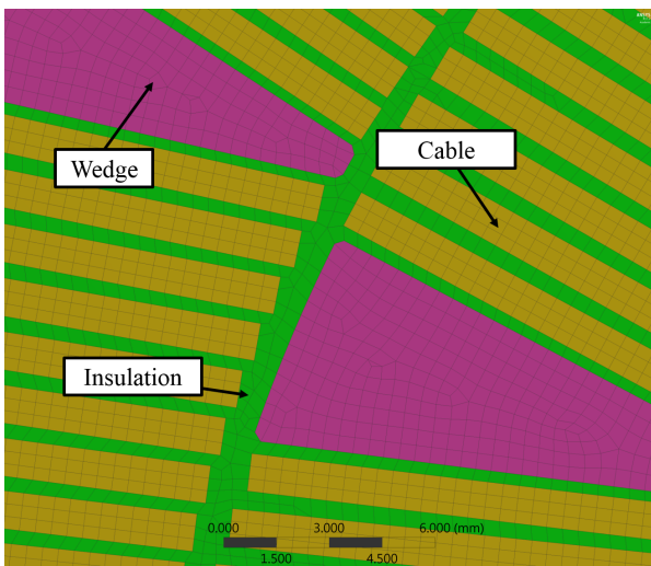
Figure C.21: Meshing used on the cable and insulation
