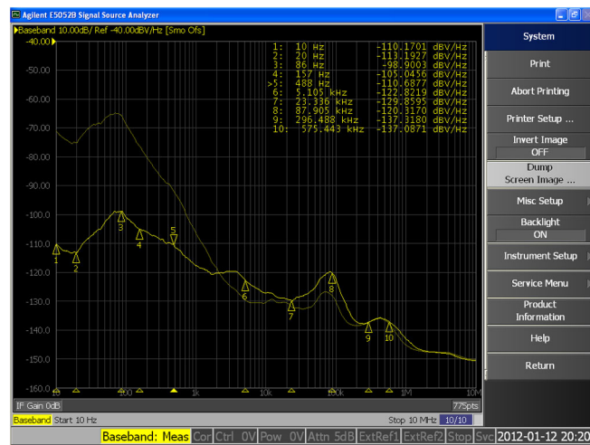
FIG. 36. Signal source analyzer screenshot illustrating the improvement of the jitter of the Nd:YLF laser: Using the in-house built synchronization unit with gain optimized within the controller bandwidth, the laser exhibits a jitter of 45 fs in the spectral range between 10 Hz and 10 MHz (bright yellow curve with arrows). For comparison, the original synchronization box results in a jitter of about 600 fs in the same spectral range (pale yellow curve).
