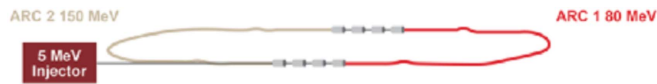
Figure 10. The facility is designed in a modular way. This picture shows a Step 1 layout of two parallel cryomodules to achieve \sim 75 MeV acceleration per linac and a final beam energy of 155 MeV (or half of it with just one initial cryomodule).
