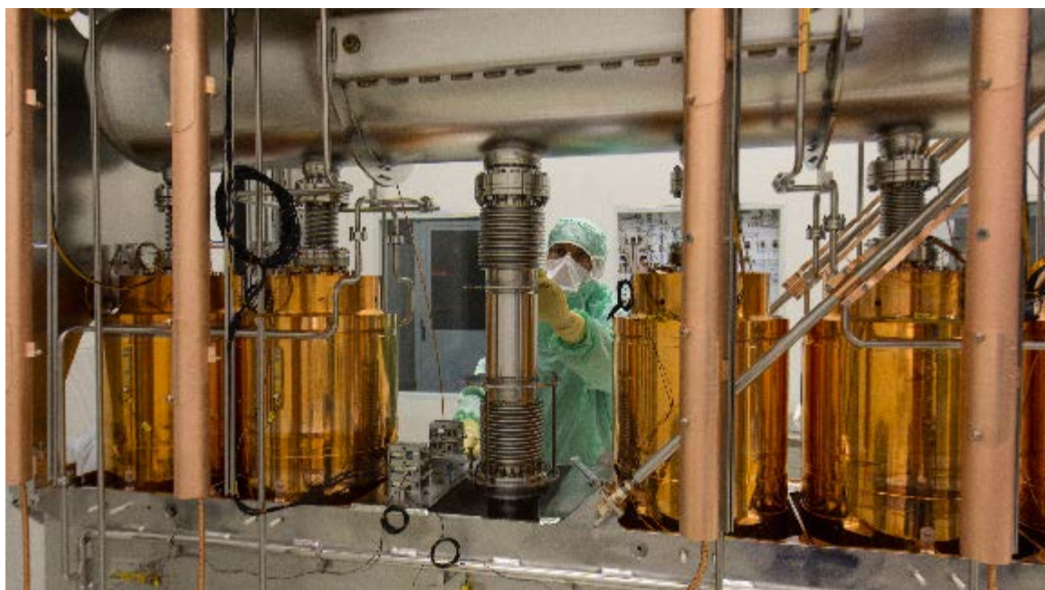
HIE-ISOLDE cryomodule with five copper RF cavities and one solenoid magnet assembled at the SM18 clean room. (Image: Maximilien Brice, CERN)
