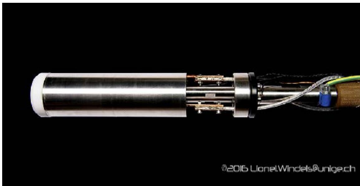
Details of the innovative superconducting coil, conceived and manufactured by researchers from UNIGE and Bruker BioSpin. (Image: © L. Windels, UNIGE)
