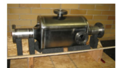
Figure 5: The three PoP cavities for cryogenic testing: a) RF dipole, b) DQW and c) 4-rod.
