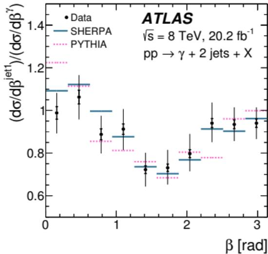
Different shape, Ratio enhanced at  $\beta = 0$  and  $\pi$  rad, in the directions towards the beams
