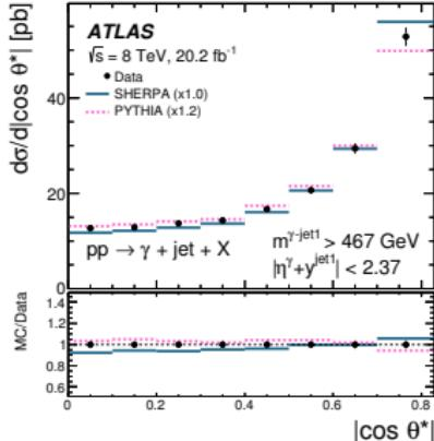
Both leading-logarithm PS MC, SHERPA and PYTHIA give an adequate description of the shape of the data, except at high  $E_T^\gamma$  and high  $m^{\gamma\text{-jet}1}$
