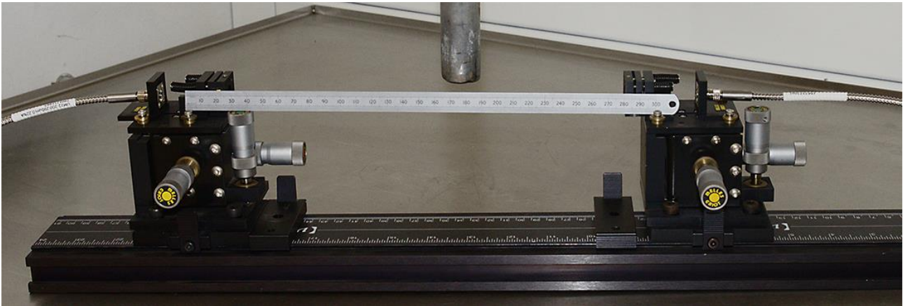
Fig. 6. Fibre test bench. The two optical fibres, connecting the remote spectrometer and light source respectively, come from left and right and light is focussed onto the fibre under test by silica lenses located within the precision manual x-y-z stages. The 60 Co radioactive source, when exposed, is located at the bottom of the steel tube seen in the centre of this photograph. The fibre under test is placed in a holder (not shown) located in the gap between the stages.
