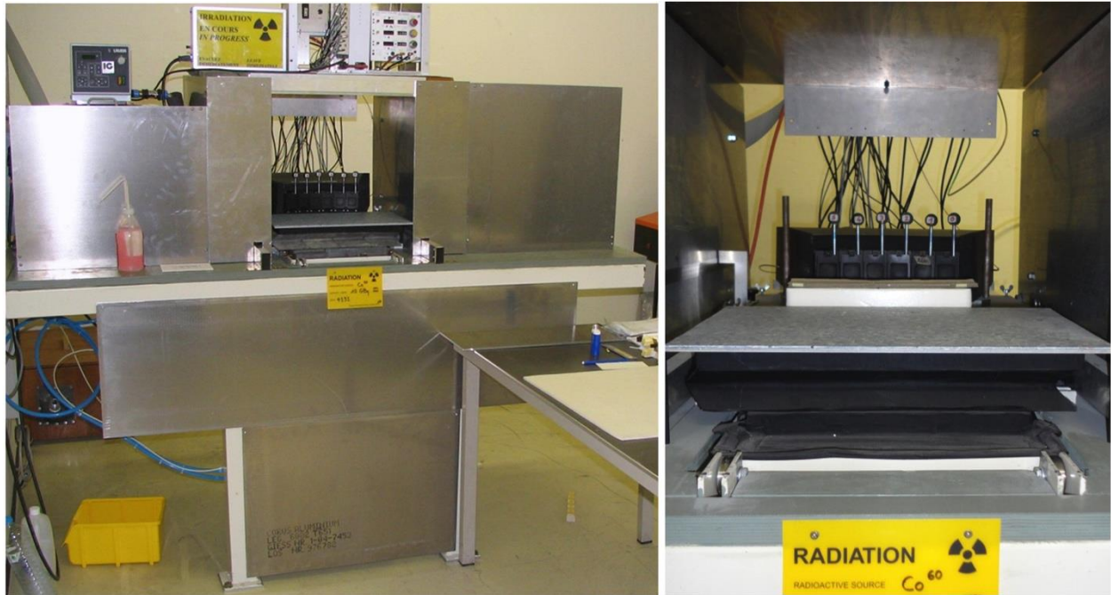
Fig. 7. Pictures of the ^{60}\text{Co} radioactive source used for studies of radiation hardness.
