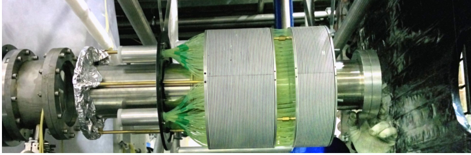
Figure 36. Picture of the IRC during installation, prior to wrapping for light tightness. The upstream and downstream modules are clearly visible with the beam incident from the right.
