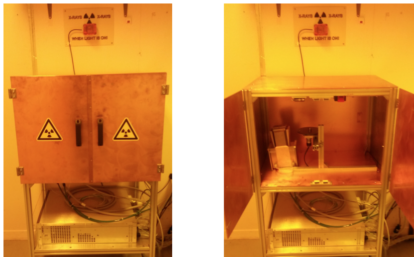
Figure 4: Custom-made shielding box containing the X-ray tube. The power supply is placed below the shielding box.
