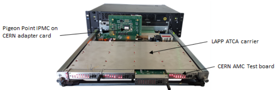
Figure 5. Test setup using LAPP ATCA test blade.
