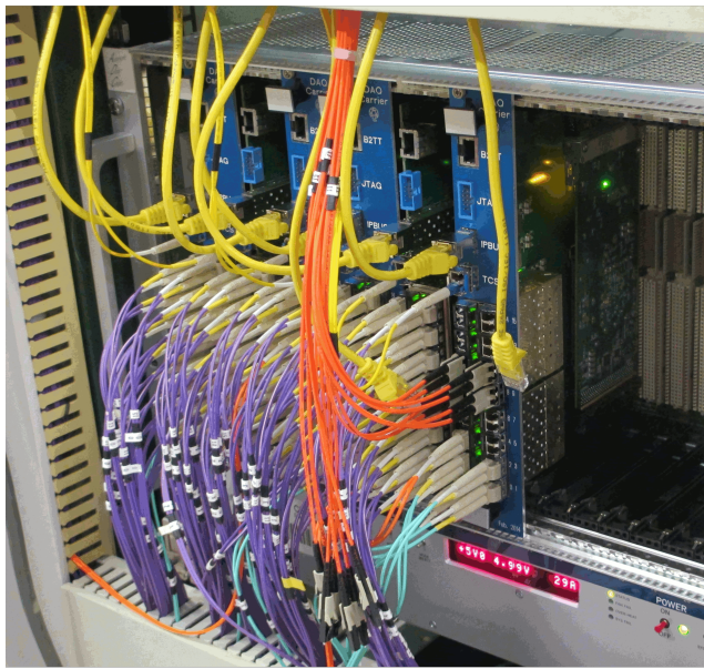
Figure 2. Five DAQ units in a VME crate (left) and more detailed view of one unit consisting of DAQ carrier card and DHCxx module (right).
