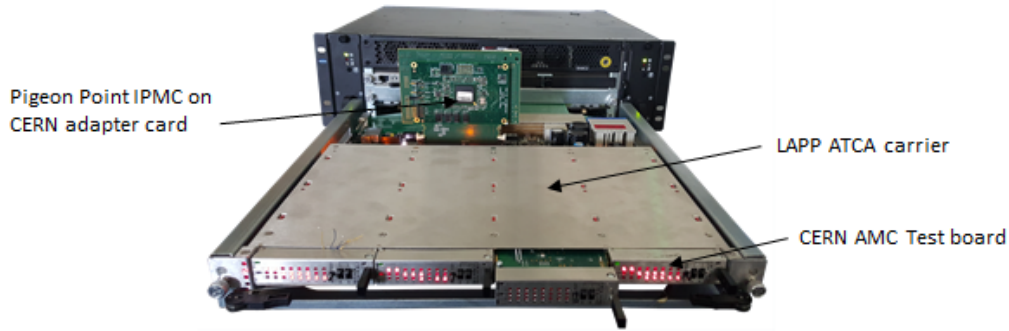
Figure 7. Test setup using the IPMC adapter card on an ATCA test blade.
