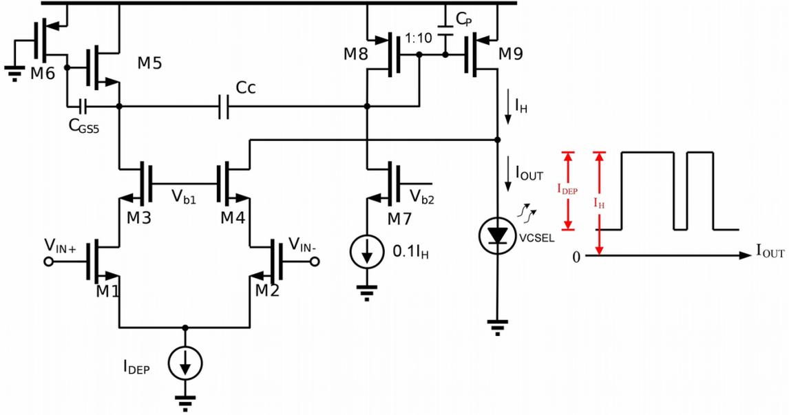
**Figure 4.** Output driver with the feedforward compensation.
