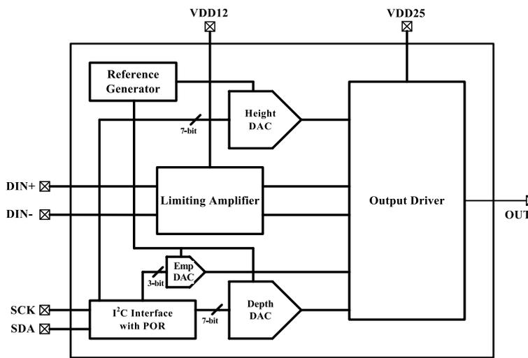
**Figure 2.** GBLD10+ block diagram.
