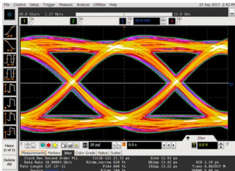
Figure 7. 10 Gb/s electrical eye diagram at 400 mV input swing.
