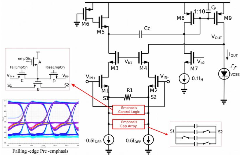
Figure 5. Configurable edge pre-emphasis in output driver.
