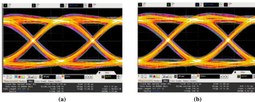
Figure 8. 10 Gb/s electrical eye diagram at different input swings: (a) 200 mV input swing; (b) 1.2 V input swing.
