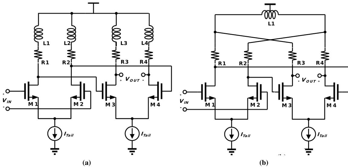
**Figure 3.** Limiting amplifier topologies: (a) traditional inductor peaking topology; (b) shared-inductor peaking topology.
