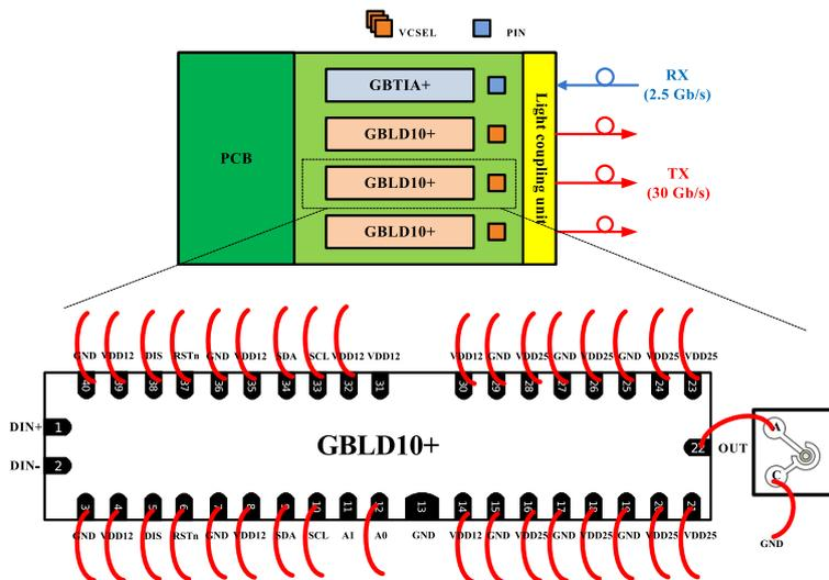
**Figure 1.** Transceiver module with three GBLD10+ and one GBTIA+.
