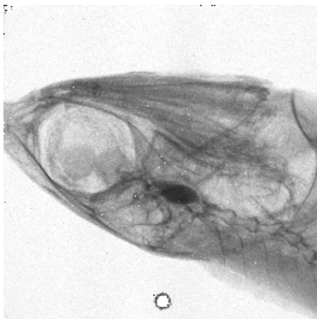
Figure 7. Image of a dried fish taken using a TSV processed Medipix3 chip connected to a 300 \mu\text{m} thick Si sensor
