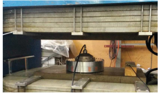
Fig. 3. 1-port reflection measurement setup in aperture of H-dipole magnet.
