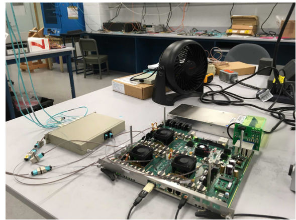
Fig. 6. Test stand of the gFEX and FELIX integration test. The gFEX prototype v2 is on the test bench at the near end, while the FELIX is installed in the PC at the far end
