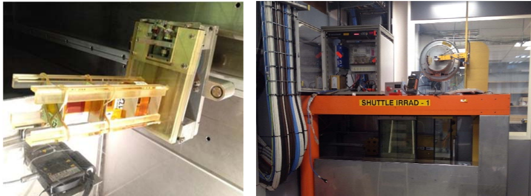
Figure 4. IRRAD1 Shuttle. Samples holder (left-hand side). Loading station (right-hand side).
