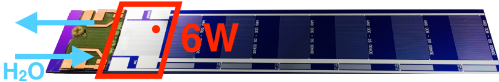
Figure 4. A 540\ \mu\text{m} thick silicon ladder with an integrated micro-channel cooling circuit. The micro-manifold is located in the end-of-ladder area, indicated with a red box in the image. The arrows indicate the approximate locations of the inlet and outlet channels. The resistive circuit are visible as grey areas.
