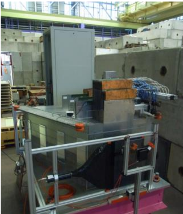
Figure 8: partly equipped EUDET steel absorber stack, with copper cooling elements for the front end electronics visible on top of the setup.
