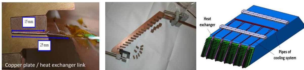
Figure 5: (Left) Design of connection of heat exchangers with one copper drain extremity (Middle) heat exchanger for 15x2 connections (Right) location of cooling system on one SiW-ECAL barrel module.
