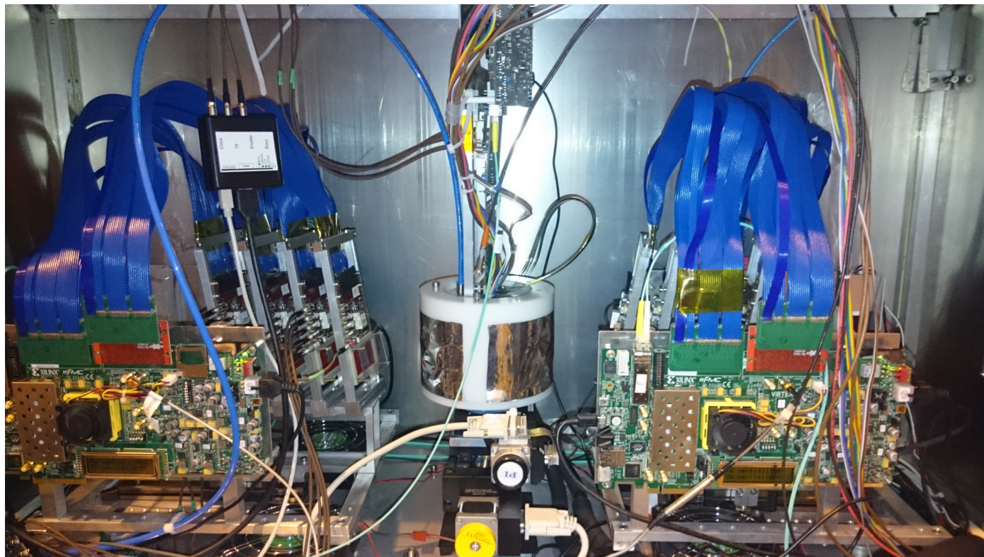
TimePix3 Telescope: Providing projected track positions and timing information
