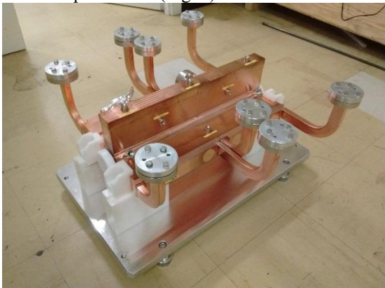
Figure 2: New SAS mock-up, after brazing and fiducialisation.
