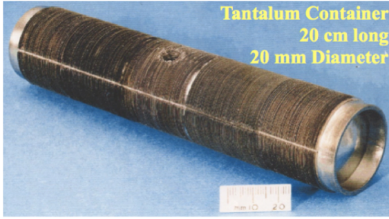
Rutherford RIST ISOL target Stacks of Ta discs and washers
